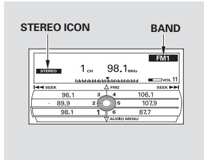
The ignition switch must be in the ACCESSORY (I) or the ON (II) position. Press the AUDIO button to view the audio control display. Turn the system on by pressing the power/volume knob or the FM/AM button. Adjust the volume by turning the power/volume knob.
