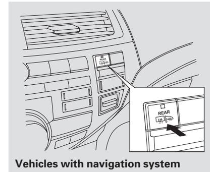
The defogger and antenna wires on the inside of the rear window can be accidentally damaged. When cleaning the glass, always wipe side to side.
