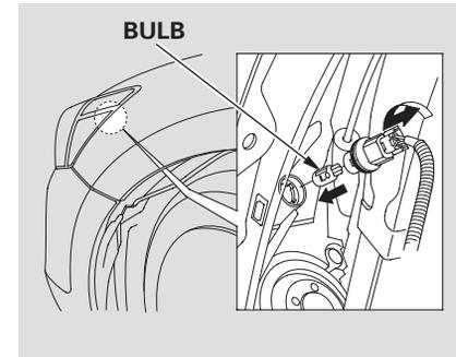
3. Remove the socket from the headlight assembly by turning it one-quarter turn counterclockwise.
