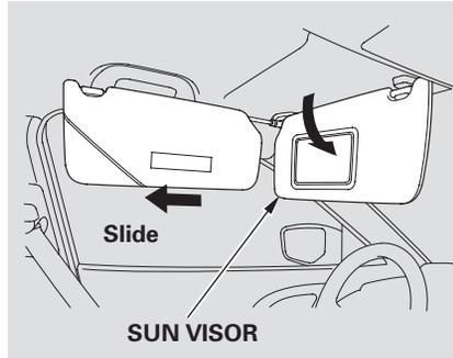
To use the sun visor, pull it down. When using the sun visor for the side window, remove the support rod from the clip, and swing it out. In this position, the sun visor can be adjusted by moving it on its slider. Do not use the extended sun visor over the inside mirror.
