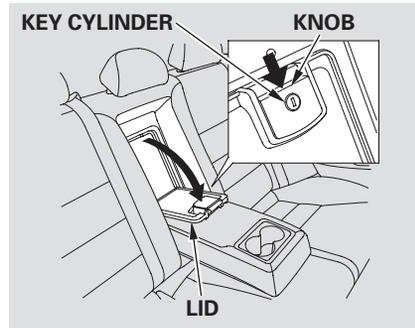
The trunk pass-through cover can be opened from inside the vehicle; it folds down onto the center armrest. Open the cover by sliding the knob downward and pulling on the cover. To close the cover, swing it up and push firmly on the top. Make sure it latches properly.
