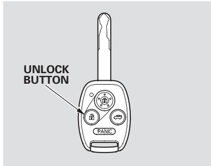
You can open all of the windows and the moonroof (if equipped) from the outside with the remote transmitter.
