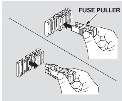
4. Check the smaller fuses in the under-hood fuse box and all the fuses in the interior fuse boxes by pulling out each one with the fuse puller provided on the back of the under-hood fuse box cover.
