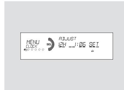
10. To enter the clock setting, turn the selector knob to select "SET," then press the knob. The display will return to the menu item display.
