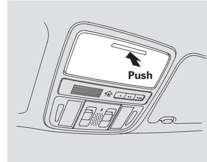
To open the sunglasses holder, push then release the indent. It will unlatch and swing down. To close it, push it until it latches. Make sure the holder is closed while you are driving.
