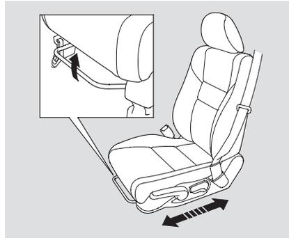
To adjust the seat forward or backward, pull up on the bar under the seat cushion's front edge. Move the seat to the desired position, and release the bar. Try to move the seat to make sure it is locked in position.
