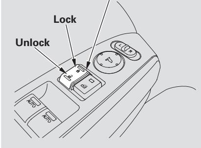
To lock all doors, push the front of the master door lock switch on either front door, pull the lock tab rearward on the driver's door, or use the key on the outside lock on the driver's door.
