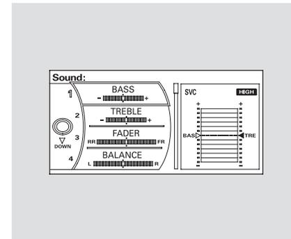
You can also adjust the sound by pushing the SOUND button repeatedly. Each mode is shown in the center display as it changes. Turn the power/volume knob to adjust the setting to your liking. When the level reaches the center, you will see “C” in the display. The system will return to the audio playing mode in the center display about 10 seconds after you stop adjusting a mode.
