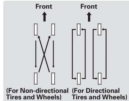
To help increase tire life and distribute wear more evenly, rotate the tires according to the maintenance messages displayed on the information display. Move the tires to the positions shown in the illustration each time they are rotated. If you purchase directional tires, rotate only front-to-back.
