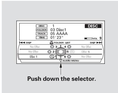
You can select any type of repeat and random modes by using the interface dial. Push the AUDIO button to display the audio information on the screen, then scroll down by pushing down the selector to select the audio menu.
