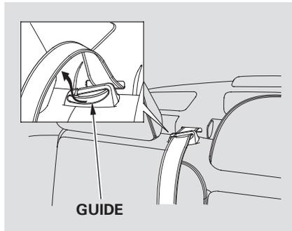
When storing cargo, you can move the rear center shoulder belt out of the way by removing the belt from the guide.
