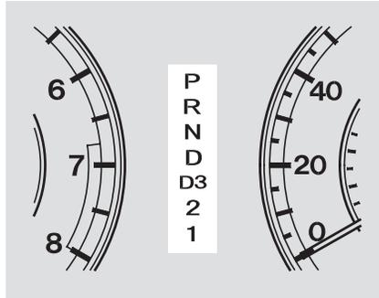
These indicators between the tachometer and speedometer show which position the shift lever is in.
