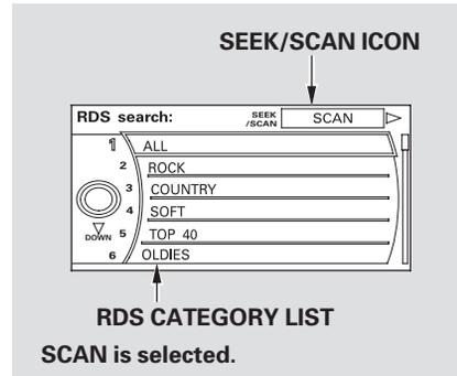
To activate RDS program scan with the interface dial, push the AUDIO button to display the FM radio information on the screen. Push the selector down, and turn the knob to select RDS SEARCH icon. Press ENTER on the selector. The screen shows you the RDS category list.
