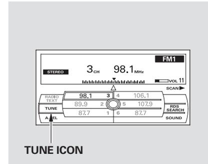
**TUNE** — Use the TUNE bar to tune the radio to a desired frequency. Press the right side of the bar to tune to a higher frequency, or the left side to tune to a lower frequency. To tune with the interface dial, push the selector down, and turn the knob to TUNE icon. Then press ENTER on the selector, and turn the knob to the desired frequency. To exit the TUNE mode, press ENTER on the selector.
