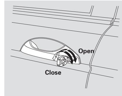
You can open and close the windows and the moonroof (if equipped) with the key in the driver's door lock.
