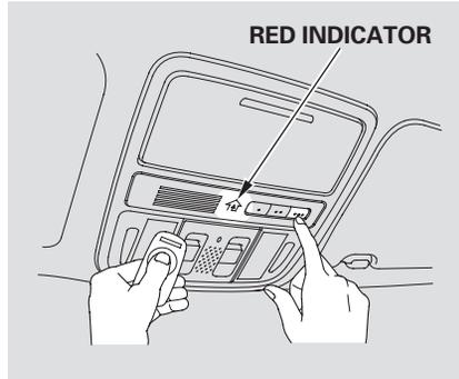
2. Press and hold the remote transmitter button and one of the HomeLink buttons at the same time.
