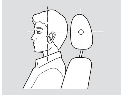
Adjust the driver's head restraint so the center of the back of your head rests against the center of the restraint.
