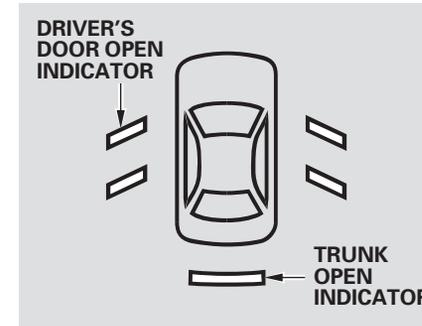
The appropriate indicator comes on in this monitor if the trunk or any door is not closed tightly.
