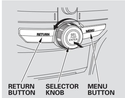
Most audio system functions can be controlled by standard buttons, bars, and knobs. In addition this, you can access some functions by using the selector knob on the audio system.
