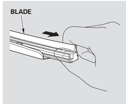
3. Remove the blade from its holder by grabbing the tabbed end of the blade. Pull firmly until the tabs come out of the holder.
