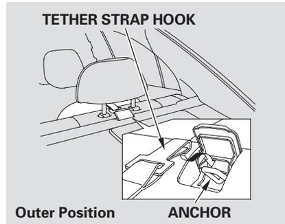
1. After properly securing the child seat (see page 44), lift the head restraint, then route the tether strap through the head restraint legs.
