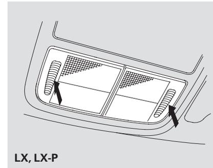
Turn on a spotlight by pushing the lens. Push the lens again to turn it off. You can use the spotlights at all times.
