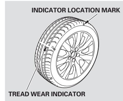
Your tires have wear indicators molded into the tread. When the tread wears down, you will see a 1/2 inch (12.7 mm) wide band across the tread. This shows there is less than 1/16 inch (1.6 mm) of tread left on the tire.
