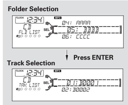
In MP3 or WMA mode, you can also select a folder or track/file from the list by using the selector knob. Push the selector knob (ENTER) to switch the display to the list displayed with three segments, then turn the knob to select a folder. Press the selector knob (ENTER) to change the display to the track/file list, then turn the same knob to select a track/file. Press the selector knob (ENTER) to set your selection.
