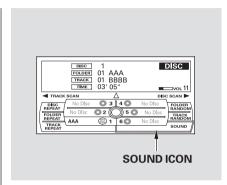
To adjust them, press the AUDIO button, push the interface selector down, and turn the interface knob to SOUND. Then press ENTER on the selector.
