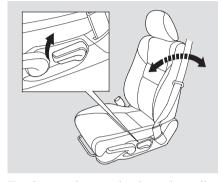
To change the seat-back angle, pull up on the lever on the outside of the seat bottom.
