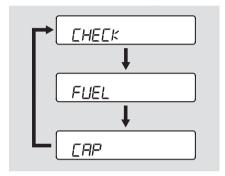
Your vehicle's onboard diagnostic system will detect a loose or missing fuel fill cap as an evaporative system leak. The first time a leak is detected a "CHECK FUEL CAP" message appears on the information display.
