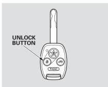
You can open all of the windows and the moonroof (if equipped) from the outside with the remote transmitter.
