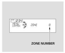
5. Once the correct zone is displayed, press the selector knob. The display then returns to normal.
