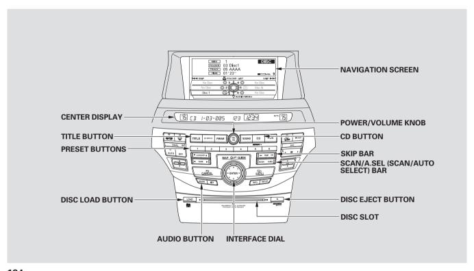
Your vehicle's audio system has an in-dash disc changer with the same controls used for the radio. To operate the disc changer, the ignition switch must be in the ACCESSORY (I) or the ON (II) position.
