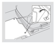
The driver's floor mat that came with your vehicle hooks over the floor mat anchors. This keeps the floor mat from sliding forward and possibly interfering with the pedals.
