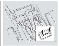
Push the right side of the switch, HI, to rapidly heat up the seat. After the seat reaches a comfortable temperature, select LO by pushing the left side of the switch. This will keep the seat warm.
