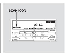
SCAN — The SCAN function samples all stations with strong signals on the selected band. To activate it, press the SCAN side of the SCAN/A.SEL bar, then release it.
