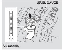
Fill the reservoir with a good-quality windshield washer fluid. This increases the cleaning capability and prevents freezing in cold weather.
