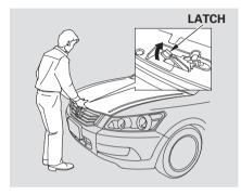
2. Reach in between the hood and the front grille with your fingers. The hood latch handle is above the "H" logo. Push this handle up until it releases the hood. Lift the hood.
