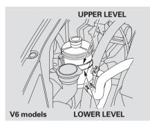
Pour the fluid slowly and carefully so you do not spill any. Clean up any spills immediately; it could damage components in the engine compartment. Always use Honda Power Steering Fluid. You may use another power steering fluid as an emergency replacement, but have the power steering system flushed and refilled with Honda PSF as soon as possible.
