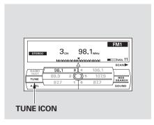
TUNE — Use the TUNE bar to tune the radio to a desired frequency. Press the right side of the bar to tune to a higher frequency, or the left side to tune to a lower frequency. To tune with the interface dial, push the selector down, and turn the knob to TUNE icon. Then press ENTER on the selector, and turn the knob to the desired frequency. To exit the TUNE mode, press ENTER on the selector.
