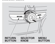
Most audio system functions can be controlled by standard buttons, bars, and knobs. In addition this, you can access some functions by using the selector knob on the audio system.
