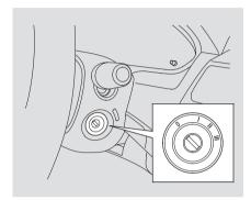
The ignition switch has four positions: LOCK (0), ACCESSORY (I), ON (II), START (III)
