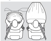
Your vehicle has a supplemental restraint system (SRS) with front airbags to help protect the heads and chests of the driver and a front seat passenger during a moderate to severe frontal collision (see page 23 for more information on how your front airbags work).
