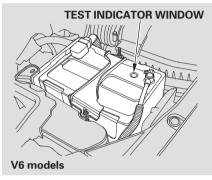
Check the terminals for corrosion (a white or yellowish powder). To remove it, cover the terminals with a solution of baking soda and water. It will bubble up and turn brown. When this stops, wash it off with plain water. Dry off the battery with a cloth or paper towel. Coat the terminals with grease to help prevent future corrosion.
