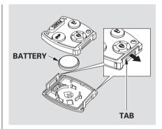
3. Inside the transmitter, separate the inner cover from the keypad by releasing the two tabs on the cover.
