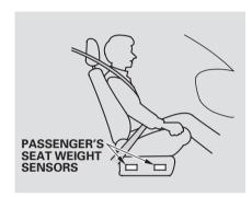
The passenger's advanced front airbag system has weight sensors under the seat. Although Honda does not encourage carrying an infant or small child in front, if the sensors detect the weight of an infant or small child (up to about 65 lbs or 29 kg), the system will automatically turn the passenger's front airbag off.
