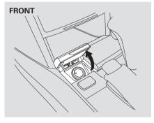
Your vehicle has two accessory power sockets; one is at the front of the center console and the other is in the console compartment.
