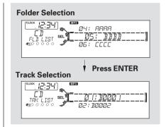
In MP3 or WMA mode, you can also select a folder or track/file from the list by using the selector knob. Push the selector knob (ENTER) to switch the display to the list displayed with three segments, then turn the knob to select a folder. Press the selector knob (ENTER) to change the display to the track/file list, then turn the same knob to select a track/file. Press the selector knob (ENTER) to set your selection.
