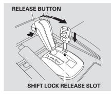
5. Push down on the key while you press the release button on the front of the shift lever and move the shift lever out of Park to neutral.
