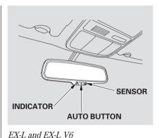
The inside mirror can automatically darken to reduce glare. To turn on this feature, press the button on the bottom of the mirror. The AUTO indicator comes on as a reminder. When it is on, the mirror darkens when it senses the headlights of a vehicle behind you, then returns to normal visibility when the lights are gone. Press the button again to turn off this feature.
