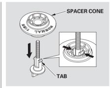
To remove the spacer cone, squeeze the tabs on the wing bolt to disengage it from the center of the spacer cone, then pull the bolt downward.
