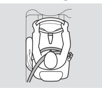
If you ever have a moderate to severe side impact, sensors will detect rapid acceleration and signal the control unit to instantly inflate either the driver's or the passenger's side airbag and activate the seat belt tensioner on the affected side.
