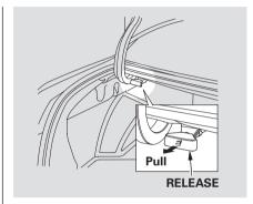
To release the seat-back from inside the trunk, pull the release under the trunk panel. Push the seat-back down from inside the trunk, or pull the seat-back down from inside the vehicle.
