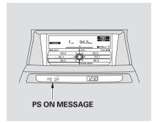
To switch the function between on and off, press and release the TITLE button. With the system on, you will see the "PS ON" message on the center display. If the station you are listening to is an RDS station, the displayed frequency switches to the station name.
