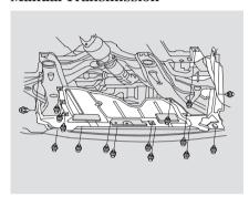
$2.4~\ell$  engine models Check the fluid level with the transmission at normal operating temperature and the vehicle sitting on level ground.
