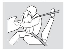
If you ever have a moderate to severe frontal collision, sensors will detect the vehicle's rapid deceleration.
