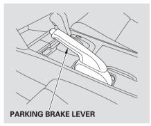
To apply the parking brake, pull the lever up fully. To release it, pull up slightly, push the button, and lower the lever. The parking brake indicator on the instrument panel should go out when the parking brake is fully released (see page 57).
