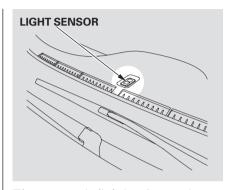
The automatic lighting feature is controlled by a sensor located on top of the dashboard. Do not cover this sensor or spill liquids on it. The automatic lighting off feature activates if you leave the headlight switch in the "FOGE" or "ED" position or if the lights are turned on by setting the switch in the "AUTO" position (if equipped), and you remove the key, then open and close the driver's door.
