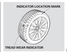
Your tires have wear indicators molded into the tread. When the tread wears down, you will see a 1/2 inch (12.7 mm) wide band across the tread. This shows there is less than 1/16 inch (1.6 mm) of tread left on the tire.
