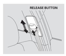
The front seats have adjustable seat belt anchors. To adjust the height of an anchor, press and hold the release button and slide the anchor up or down as needed (it has four positions). Never place the shoulder portion of a lap/shoulder belt under your arm or behind your back. This could cause very serious injuries in a crash.
