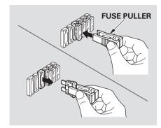
4. Check the smaller fuses in the under-hood fuse box and all the fuses in the interior fuse boxes by pulling out each one with the fuse puller provided on the back of the under-hood fuse box cover.
