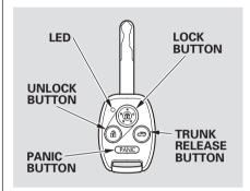
LOCK — Press this button once to lock all doors. Some exterior lights will flash once. When you push LOCK twice within 5 seconds, you will hear a beep to verify that the doors are locked and the security system (if equipped) has set. You cannot lock the doors if any door is not fully closed or the key is in the ignition switch.
