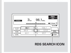
On the FM band selected, you can select the program type provided by the RDS. Press the AUDIO button to display the radio information on the screen. Push down the selector on the interface dial, then turn the knob to select RDS SEARCH icon. Press ENTER to set your selection. The principal RDS categories are shown as follows;
