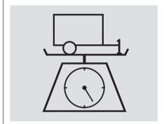
Total Trailer Weight: The maximum allowable weight of the trailer and everything in or on it must not exceed 1,000 lbs (450 kg). Towing a load that is too heavy can seriously affect your vehicle's handling and performance. It can also damage the engine and drivetrain.
