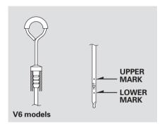
4. Remove the dipstick and check the fluid level. It should be between the upper and lower marks. 5. If the level is below the lower mark, add fluid into the dipstick hole to bring it to the level between the upper and lower marks.
