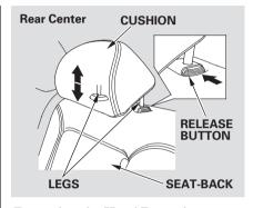
Removing the Head Restraint
