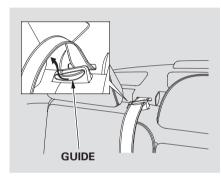
When storing cargo, you can move the rear center shoulder belt out of the way by removing the belt from the guide.
