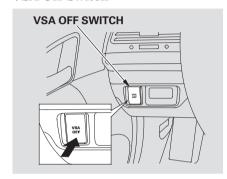
This switch is under the driver's side vent. To turn the VSA system on and off, press and hold it until you hear a beep.
