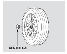
15.Remove the center cap (if equipped) before storing the flat tire in the trunk well.
