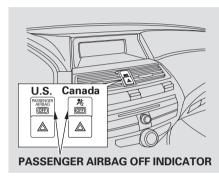
This indicator alerts you that the passenger's front airbag has been shut off because weight sensors detect about 65 lbs (29 kg) or less (the weight of an infant or small child) on the front passenger's seat. It does *not mean* there is a problem with the airbag.
