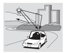
Radio signals, especially on the FM band, are deflected by large objects such as buildings and hills. Your radio then receives both the direct signal from the station's transmitter, and the deflected signal. This causes the sound to distort or flutter. This is a main cause of poor radio reception in city driving.
