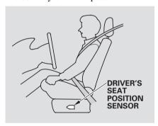
If there is a problem with the sensor, the SRS indicator will come on, and the airbag will inflate in the normal manner regardless of the driver's seating position.
