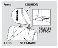
Adjusting the Head Restraint
