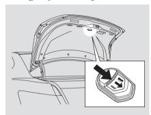
As a safety feature, your vehicle has a release lever on the trunk latch so the trunk can be opened from the inside.
