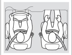
Your vehicle also has side airbags to help protect the upper torso of the driver or a front seat passenger during a moderate to severe side impact (see page 27 for more information on how your side airbags work).
