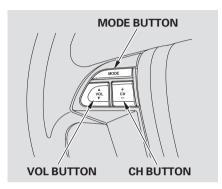
Three controls for the audio system are mounted in the steering wheel hub. These let you control basic functions without removing your hand from the wheel.
