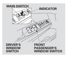
Turn the ignition switch to the ON (II) position to raise or lower any window. To open a window, push the switch down and hold it. Release the switch when you want the window to stop. Pull back on the switch and hold it to close the window.
