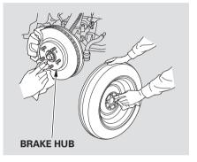
11.Before mounting the spare tire, wipe any dirt off the mounting surface of the wheel and hub with a clean cloth. Wipe the hub carefully; it may be hot from driving.
