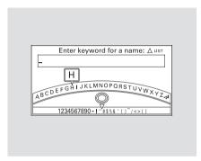
Enter the keyword for a person's name, such as the first name or last name, using the Interface Dial. If the system does not find an exact match, say or select "LIST" when you finish entering the keyword.
