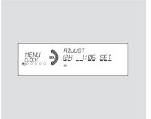
4. Turn the selector knob to select the item which you want to adjust. Turning the knob will change the selected item between the clock display setting, hours, minutes, and SET. The selected item is indicated with △ in the display.
