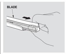
3. Remove the blade from its holder by grabbing the tabbed end of the blade. Pull firmly until the tabs come out of the holder. 4. Examine the new wiper blades. If they have no plastic or metal reinforcement along the back edge, remove the metal reinforcement strips from the old wiper blade, and install them in the slots along the edge of the new blade.
