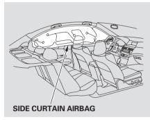
In a moderate to severe side impact, sensors will detect rapid acceleration and signal the control unit to instantly inflate the side curtain airbag and activate the seat belt tensioner on the driver's or the passenger's side of the vehicle.
