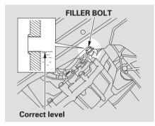
Remove the transmission filler bolt, and carefully feel inside the bolt hole with your finger.
