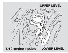
Check the level on the side of the reservoir when the engine is cold.
