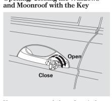
You can open and close the windows and the moonroof (if equipped) with the key in the driver's door lock.
