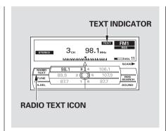
To activate radio text display, use the interface dial. Push the selector down, and turn the knob to select RADIO TEXT icon. Press ENTER on the selector to enter the setting.
