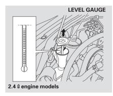
Check the level in the windshield washer reservoir at least monthly during normal use.
