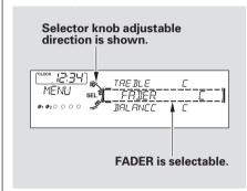
Press the MENU button to display the sound settings. Turn the selector knob to select an appropriate setting: bass, treble, fader, balance, SUBW\* (subwoofer) and SVC (speedsensitive volume compensation). Press the selector (ENTER) knob to enter the setting, then turn the selector knob to adjust the setting.
