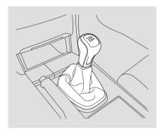
On models with manual transmission The manual transmission is synchronized in all forward gears for smooth operation. It has a lockout so you cannot shift directly from fifth to reverse.
