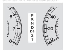
These indicators between the tachometer and speedometer show which position the shift lever is in.
