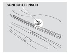
The climate control system has two sensors. A sunlight sensor is in the top of the dashboard, and a temperature sensor is next to the steering column. Do not cover the sensors or spill any liquid on them.
